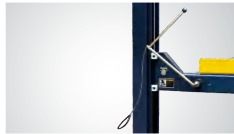
▲ Proprietary lock control system.
